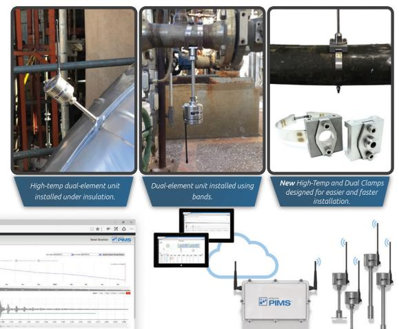
webPIMS<sup>™</sup> cloud-based data portal offers all available information including corrosion rate and temperature-corrected thickness data.
