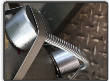
Dual-element sensor attachment can be either magnetic housing, or via strap with temporary or permanent couplant.
